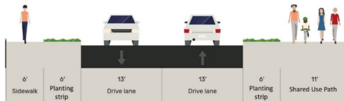
Figure 3. Section A (Monroe St to Madison St) – Proposed (26' curb to curb) *
