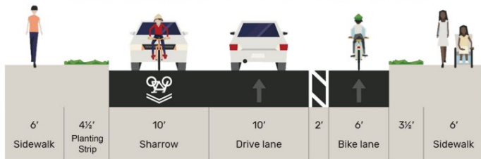
Figure 11. Section E (SE Adams St to SE 17 th St) – Proposed (28' curb to curb)
