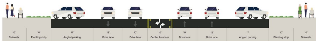
Figure 2. Section A (3 rd to 6 th , 10 th to 13 th ) – Existing (88' curb to curb)
